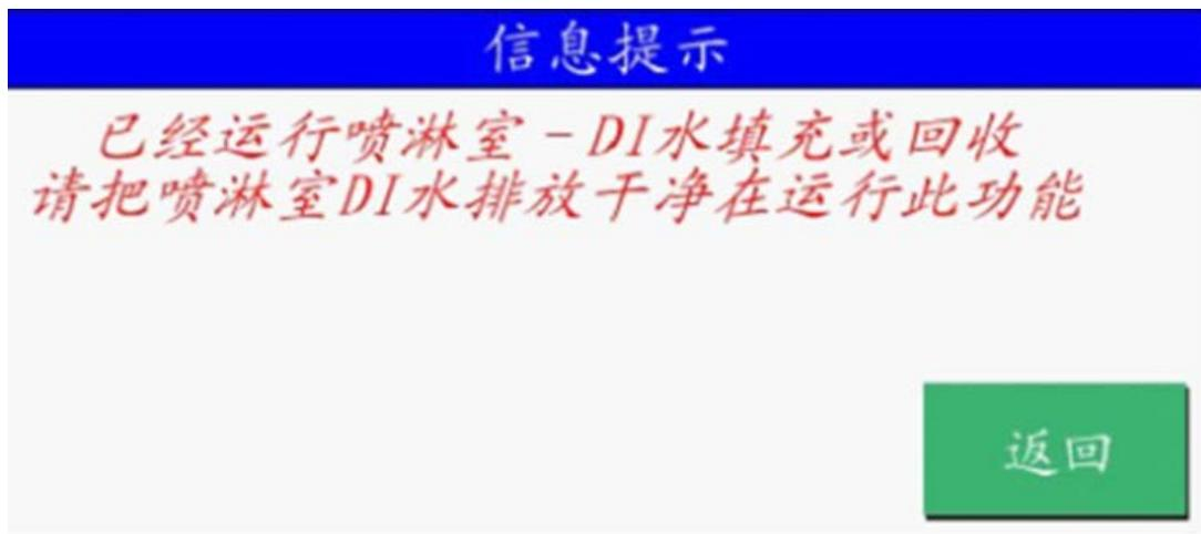
If you want to add DI water into spray tank or drain DI water from spray tank, this screen will appear and you have to enter Manual menu again.
