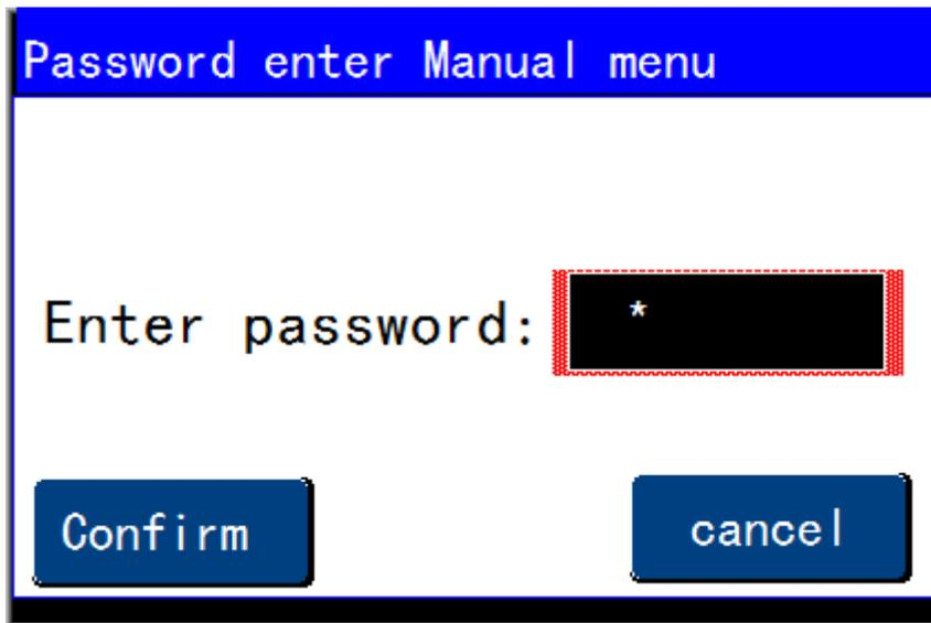
The manual password is: 2222. Input 2222 and press enter to enter into Manual Menu
