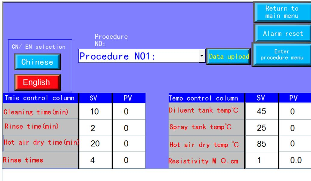
The screenshot shows a control interface with a blue background. At the top right, there are three buttons: "Return to main menu", "Alarm reset", and "Enter procedure menu". In the center, there is a "Procedure NO:" dropdown menu currently set to "Procedure N01:", with a "Data upload" button next to it. On the left, there is a "CN/ EN selection" box with "Chinese" and "English" buttons. Below this is a table with two columns: "Time control column" and "Temp control column".
