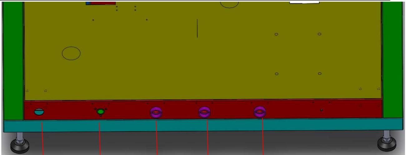
Power cable port (3 phase, AC380V 50HZ)
