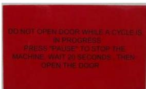
Safety reminds sign: This sign reminds you never open the front door when the machine is running. Press “pause” to stop the machine and wait for about 20 seconds and then open the door. (if have pause key)
